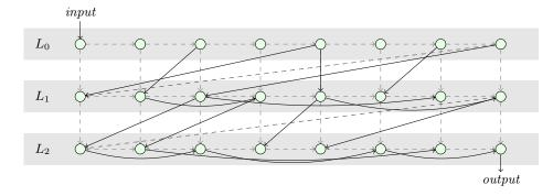
Fig. 3: The Balloon data-dependency graph on n = 8 blocks and r = 2 rounds, drawn with  $\delta = 1$  for simplicity. (The real construction uses  $\delta \ge 3$ .) The dashed edges are fixed and the solid edges are chosen pseudorandomly by applying the random oracle to the salt.
