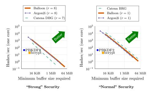
Fig. 5: The Balloon algorithm outperforms Argon2i and Catena DBG for many settings of the security parameters, and Balloon is competitive with Catena BRG. We instantiate Argon2i, Balloon, and Catena with Blake2b as the underlying cryptographic hash function.
